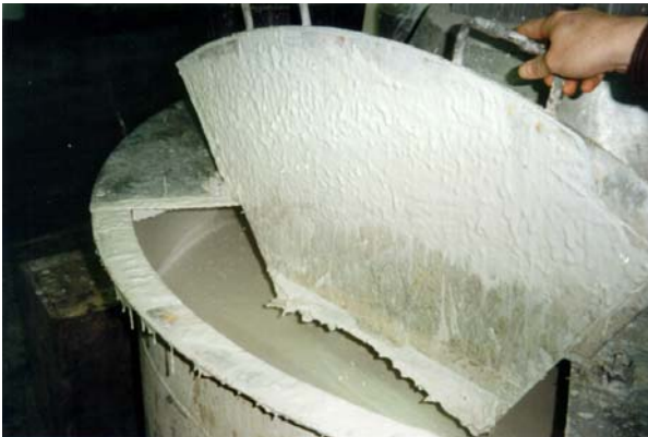
Paint vessel without coating
