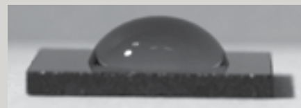
An uncoated surface repels a water drop
